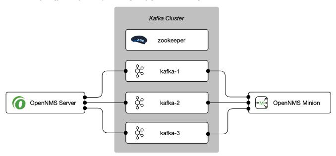
*Network topology used for the following configuration example*
